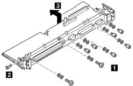
**Note:** In step **1**, each screw has a flat washer and a lock washer. When reinstalling the screws, make sure that the lock washer is placed next to the head of the screw. Incorrect washer placement can cause metal to flake.
